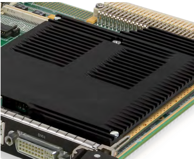
VSB2105 (Ultra-efficient heatsink for low air flow chassis)
