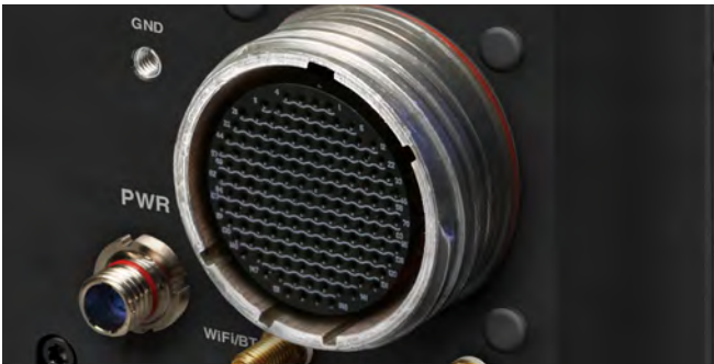
SB1002-LC (Showing rugged 38999 connector)
