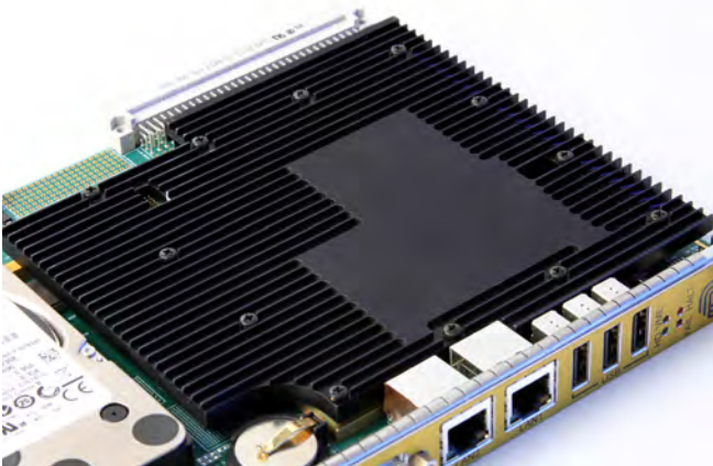
VB2105 (Ultra-efficient heatsink for low air flow chassis)
